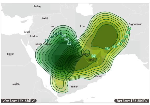
Ku/S Band Transponders: 2 x 25MHz Polarization: Linear / Circular Uplink/Downlink Frequency: 13.858 – 13.883 / 2.630 – 2.655
