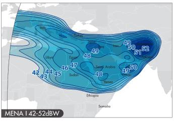
48 Ku-band Transponders (54, 72 or 108 MHz) for 5 beams Polarization: Linear (H&V)
