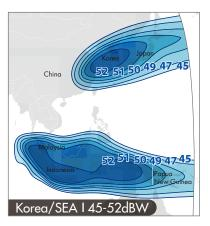
Ku-Band Transponders: 51 (49 x 54 MHz and 2 x 108 MHz) Polarization: Linear (H&V)
